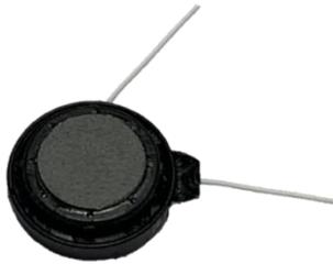
A500A ultrasonic transducer is designed to deliver outstanding performance at around 500 kHz frequency using our in-house piezoceramic and acoustic matching layer along with state-of-art technologies. The transducer works as a signal transmitting and receiving unit. This ultrasonic transducer is suitable for gas flow detection and proximity measurement with precise control as well as extraordinary reliability.
