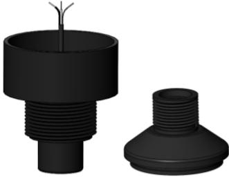
A150E works as a signal transmitting and receiving unit. This ultrasonic transducer is suitable for non-contact level detection and proximity measurement. In particular, the transducer with the PVDF housing can operate under harsh chemical environment to measure the level of fluids, pastes, and coarse bulk materials.
