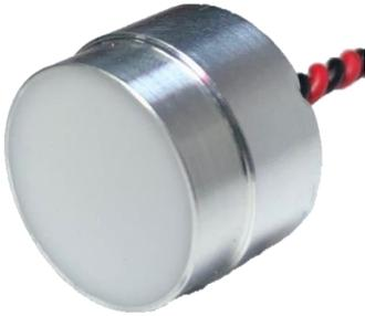
A150A ultrasonic transducer is designed to deliver outstanding performance at around 150 kHz frequency. The transducer works as a signal transmitting and receiving unit. This ultrasonic transducer is suitable for proximity measurement, web guiding control, non-contact level measurement and robotics, etc.
