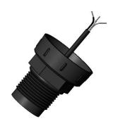
A150C works as a signal transmitting and receiving unit. This ultrasonic transducer is suitable for non-contact level detection and proximity measurement. In particular, the transducer with the PVDF housing can operate under harsh chemical environment to measure the level of fluids, pastes, and coarse bulk materials.
