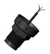
A125C works as a signal transmitting and receiving unit. This ultrasonic transducer is suitable for non-contact level detection and proximity measurement. In particular, the transducer with the PVDF housing can operate under harsh chemical environment to measure the level of fluids, pastes, and coarse bulk materials.
